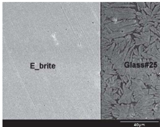
Fig. 6 Scanning electron micrograph of the bonding interface between E-brite and glass No. 25 after 4 h at 850 °C
